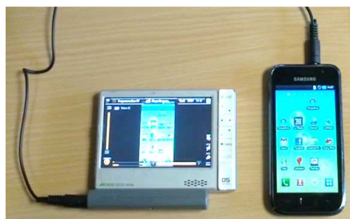
Figure 1. A simple portable set-up to record the audio-video flux on Android-based smartphones
